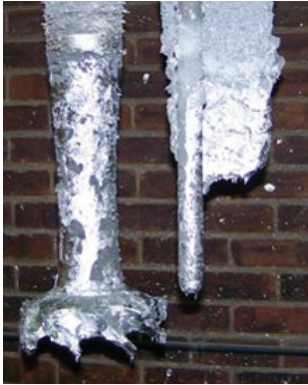
Worn graphite rotor replaced after just 300 degassing cycles.
