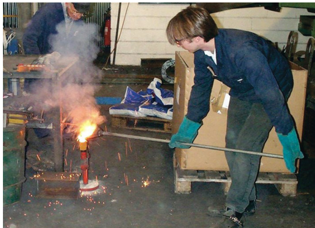
A small ladle bowl is used to collect and pour a metal sample.
