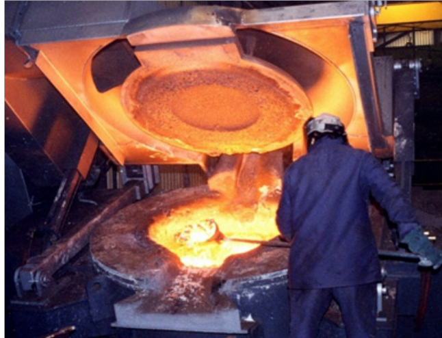
A large ladle bowl effectively removes slag from an induction furnace.
