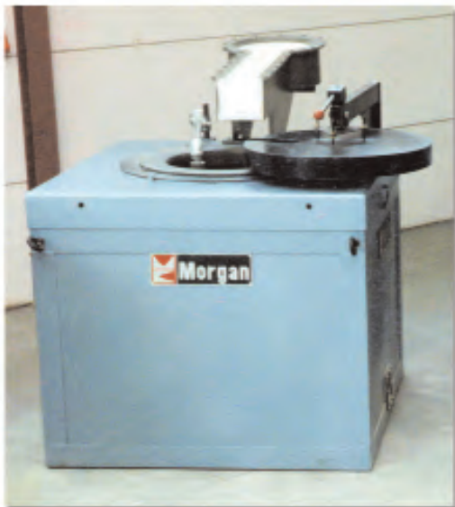
▲ Morgan's Electric Resistance Bale Out Furnace.
