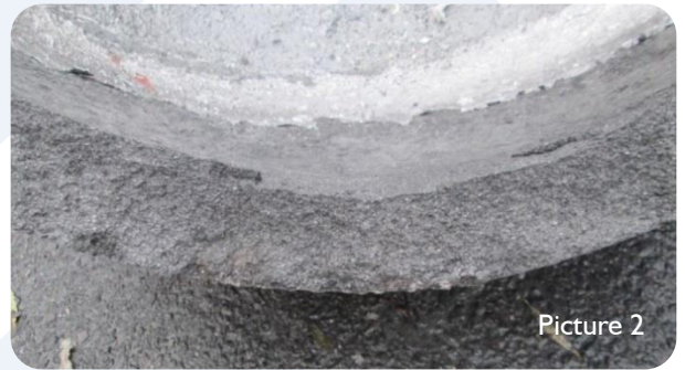
Picture 2 TopAl LTP, no bottom oxidation after 13 months of use
