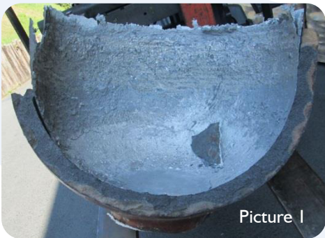
Picture 1 Existing Crucible after 7 months
