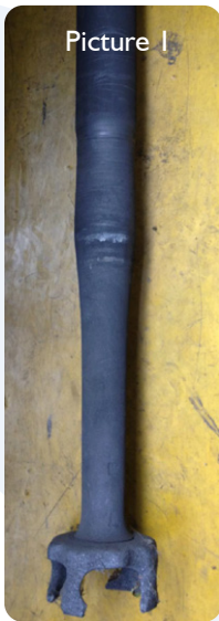
Picture 1 Existing Rotor after 100 treatment cycles.
