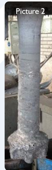
Picture 2 DGRU I50-700-S02T2 after 1700 treatment cycles.
