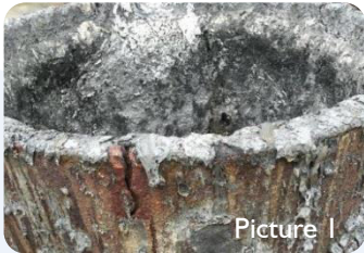
Picture 1 Existing Crucible after 42 days.
