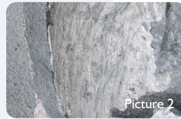
Picture 2 TPS 587 TopAl STAR Coating after 154 days.
