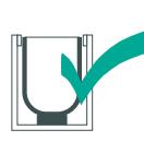
Ceramic fibre blanket should be used for sealing/packing the top edge in bale-out and some tilting furnaces.
