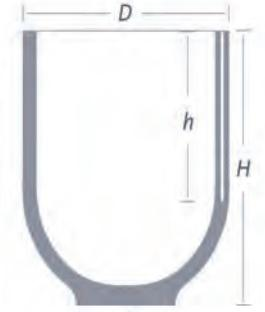
Product shapes BN & NO are available with or without Pyrometer-pocket (PT)/Pyrometer-hole (PL)
