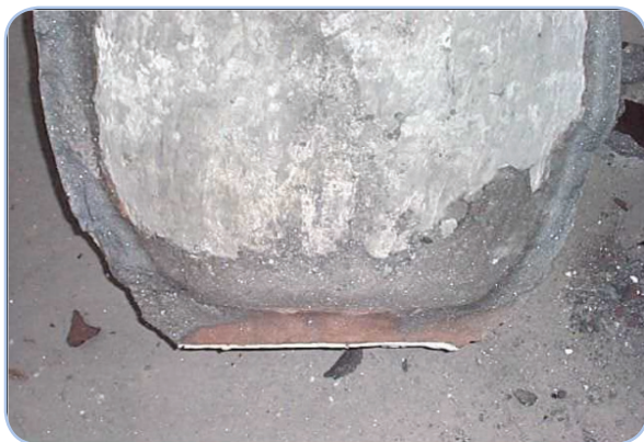
Crucible Base oxidation caused by using ceramic fibre as a parting medium between the crucible and base.
