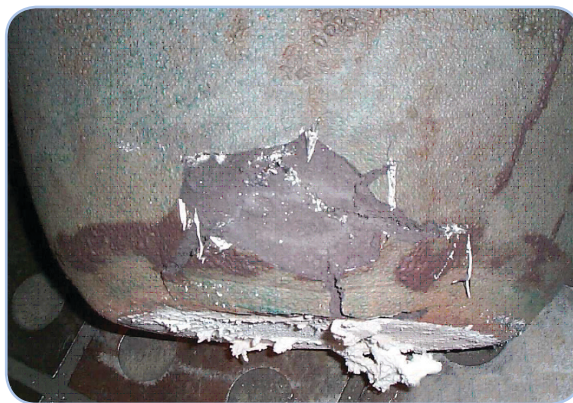
Crucible Base oxidation caused by using ceramic fibre as a parting medium between the crucible and base.
