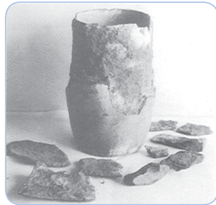
The effect of heating a wet crucible too quickly
