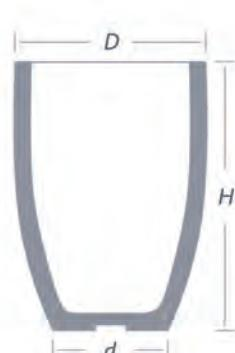
Cut-out (AE) up to D=615: 40 x 80 (H x D in mm)
