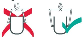
Basket tongs must hold the crucible on its lower third for lifting.
