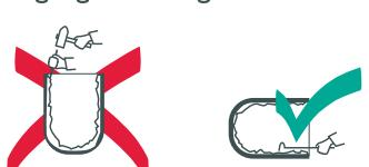
The crucible should be cleaned out by careful scraping while it is still red hot.
