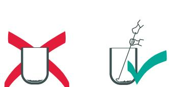
The crucible must be emptied before switching off the furnace.
