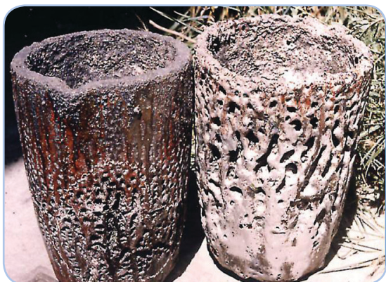
Fig. 3 – Metal with a high flux concentration was allowed to overflow these crucibles, eating away the exterior surface.
