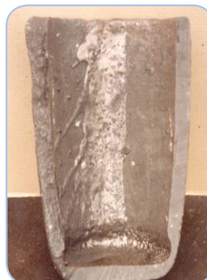
Fig. 3 – Metal with a high flux concentration was allowed to overflow these crucibles, eating away the exterior surface.
