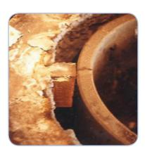
Figure 3. Gripping blocks located too close to the top of the crucible produced a vertical crack.
