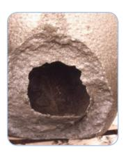
Figure 7. The impact of charge material dropped into the crucible produced this damage.
