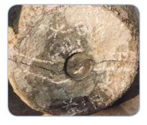
Figure 6. Thermal stress caused this crack extending across the bottom of the crucible.
