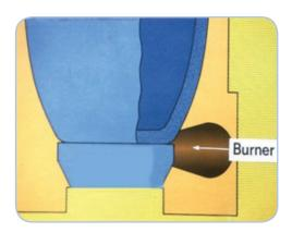
Figure 2. Crucible mounted on a properly positioned base.
