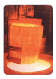
Figure 5. Lifting shanks must be properly sized for your crucible and must provide adequate support.
