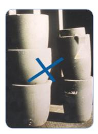
Figure 1. Improper stacking will damage crucibles.
