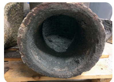
The erosion from the metal flow resulting in thinning of the crucible lining.
