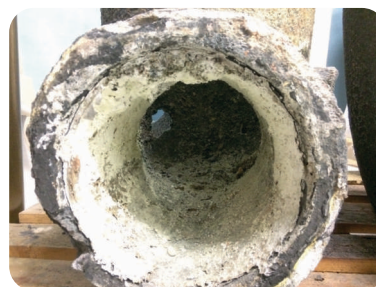
The crumbling of the material indicating oxidation on the boss.
