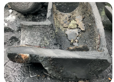
No signs of erosion or significant oxidation are visible.
